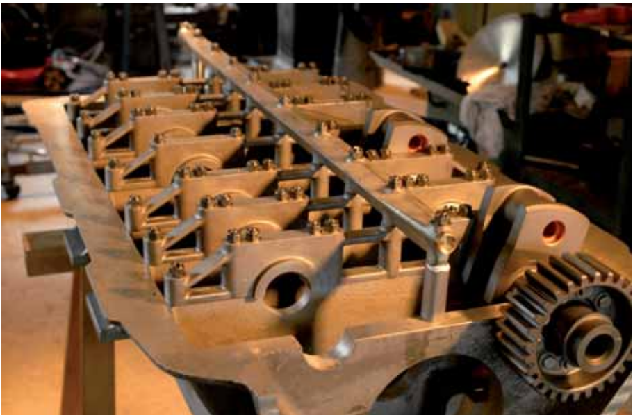
The new crankcase, inverted, with its crankshaft, bearing caps, and central oil gallery.
